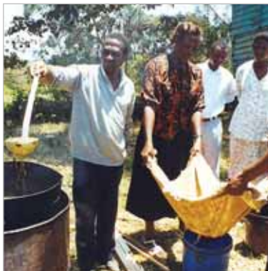
9.8 Using a ladle to transfer the water and molten beeswax mixture into a piece of hessian sacking Tanzania © NB
