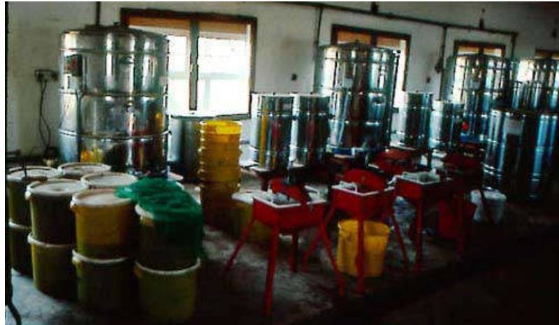
Figure 2.6 : Honey presses in the foreground and water jacketed settling tanks in the background at the honey processing centre of Northwestern Bee Products, Kabompo, Zambia, which buys, processes and exports
