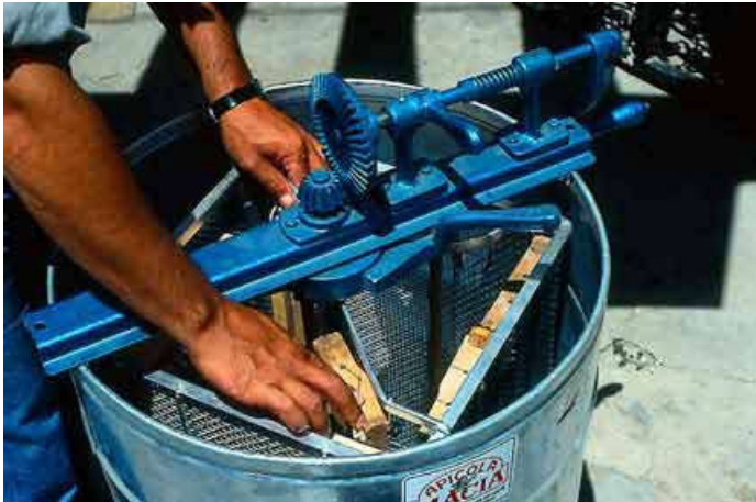
Figure 2.10: Manual 4 frame radial (medium size super frames), 4 frame tangential (2 deep and 2 medium size super frames) and comb honey extractor all in one made from construction steel, bicycle parts, 110 litre plastic drum and 5-mesh galvanized screen. This is a beekeeper's design (Mr Beizel, Formosa, Argentina) adopted and modified during an FAO sponsored beekeeping project
