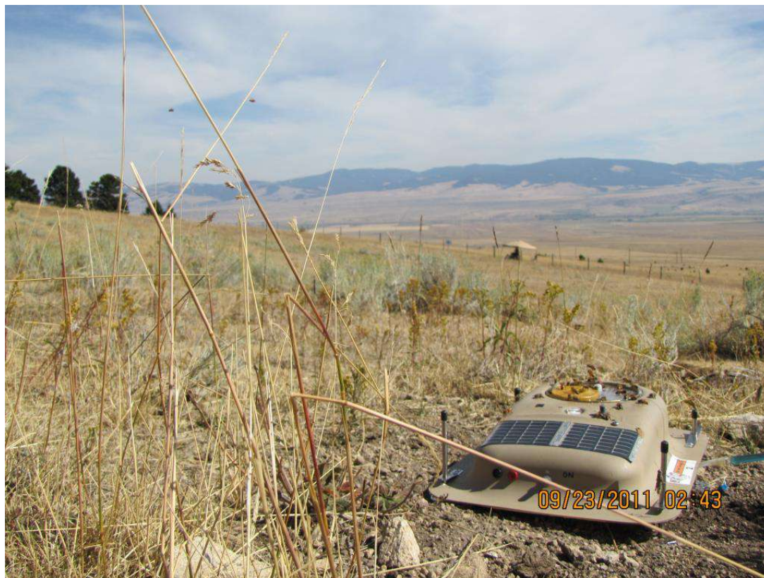
Figure 2. Solar-powered, micro-processor-controlled bee-conditioner system with scent and reward (proprietary syrup solution) dispensing systems. Reward intervals can be controlled automatically by the device, re-programmed as needed, or remotely controlled by wireless communications.
