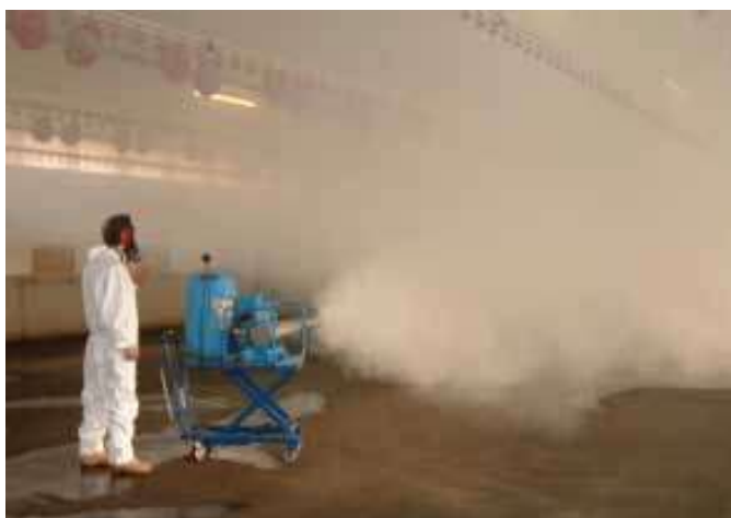
Figure 5 : Biocidal treatment of an empty barn by thermonebulisation. The insecticide solution is sprayed in fine droplets which ensures a wide aerial distribution of the substance [26].
